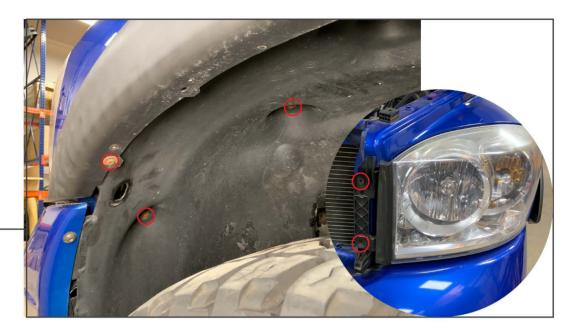
Remove the (3) 8mm screws securing the fender liner to the vehicle. Fold back the fender liner to access the nut securing the headlight to the vehicle. Then remove the (2) 10mm bolts from the front of the headlight. Pull the headlight away from the vehicle.
