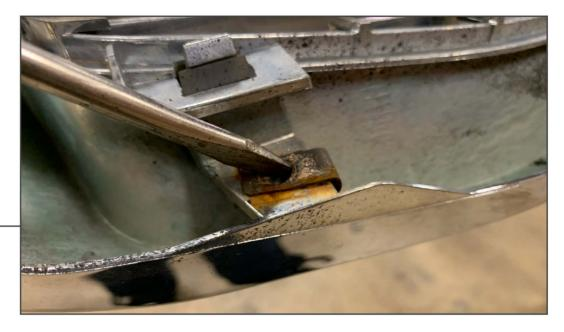
Transfer the (6) clip nuts from the factory grille onto the new grille.
