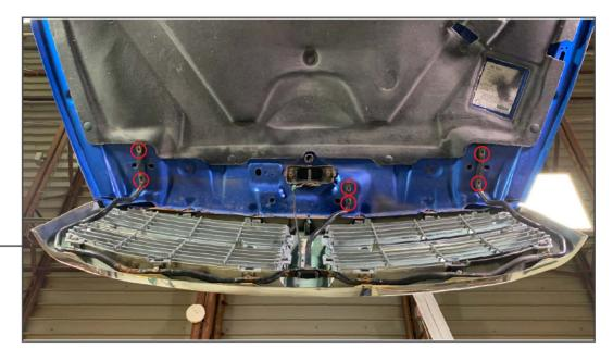
Using the same 8mm socket, remove the (6) bolts securing the grille brace to the underside of the hood.
