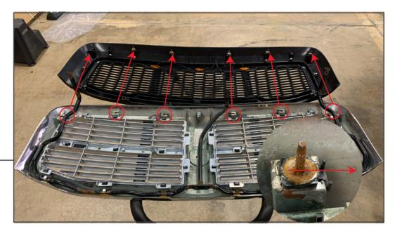
Transfer the (6) clip stud fasteners across the top of the grille onto the new grille.
