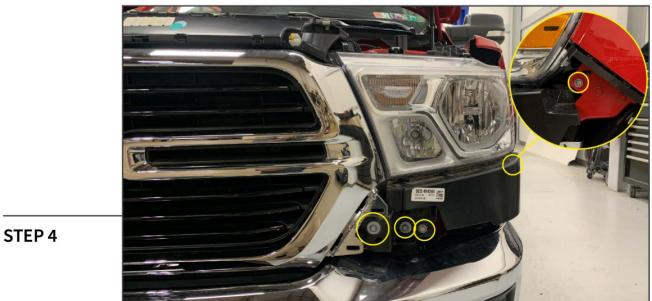
Remove (4) 10mm bolts from below the headlight assembly.
