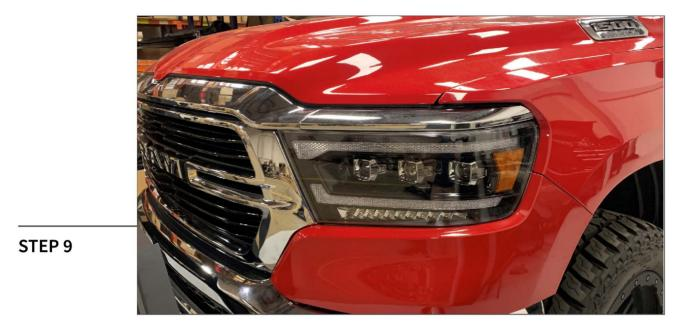
Plug the headlight into the vehicle harness and the previously routed DRL harness. Begin re-assembling the vehicle following steps 1-6 in reverse order.
