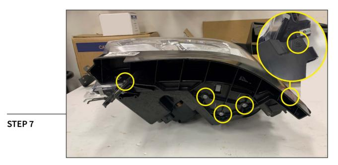
Remove (5) T-25 Torx screws from the lower plastic panel on the headlight. Remove the plastic panel from the headlight. Transfer the plastic panel and hardware to the new LED headlight.
