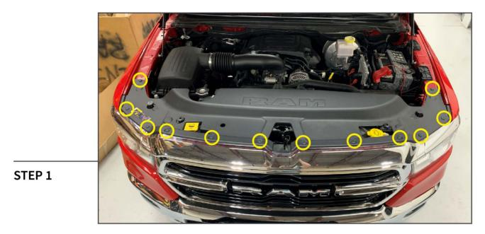
Open the hood. Remove (12) plastic push clips from the radiator support cover. Remove cover from vehicle.
