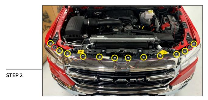
Remove (12) 10mm bolts, and (2) plastic push clips from the upper chrome panel. Remove the upper chrome panel from the vehicle.
