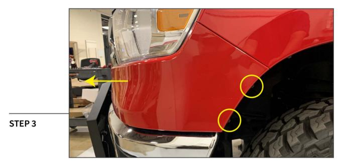
Remove (2) 8mm screws from the inner fender above the front bumper. Peel the plastic panel outward from the fender, then gently pry the front of the panel away from the vehicle.
