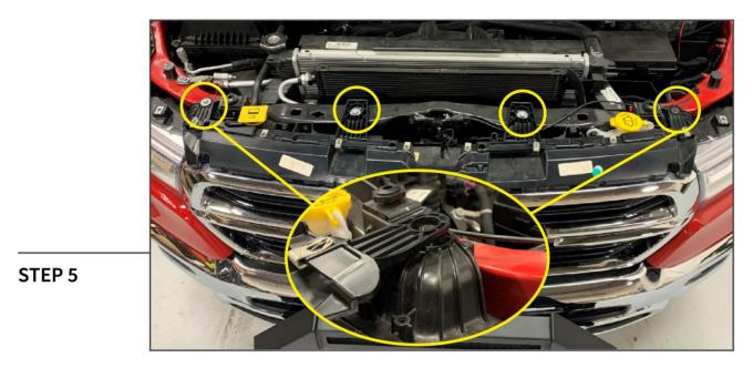
Remove (4) 10mm bolts from the top of the grille . Slightly lift the grille tabs over the bolt holes, then remove the grille from the vehicle.
