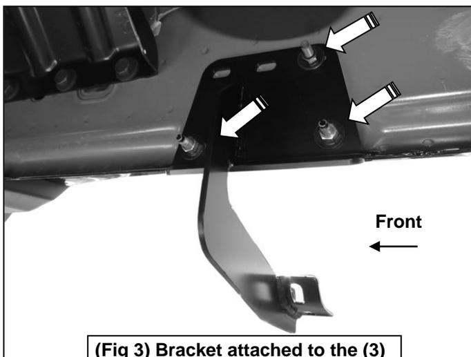
(Fig 3) Bracket attached to the (3) front studs on the passenger side
