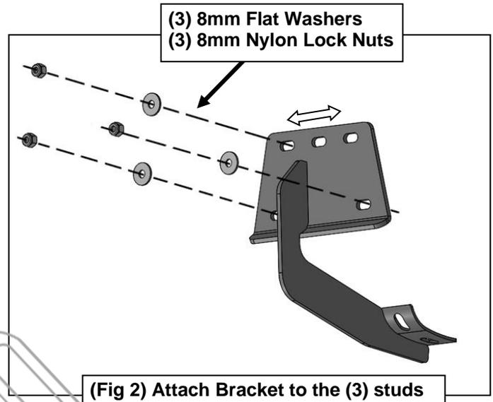
(Fig 2) Attach Bracket to the (3) studs
