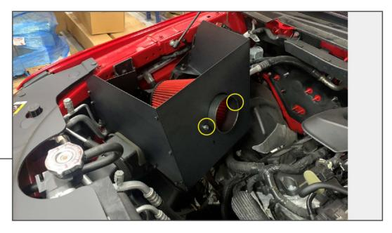
Place the heat shield into the vehicle at the original air box location. Ensure all (4) rubber grommets are in the vehicle pegs. Install the air filter adapter onto the air filter and tighten the supplied air filter clamp. Install the adapter into the heat shield using (2) M6x1.00 x 12mm bolts, (2) M6 lock washers, and (2) M6 flat washers.
