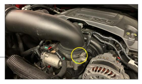
Loosen the intake hose at the throttle body using a 8mm socket.
