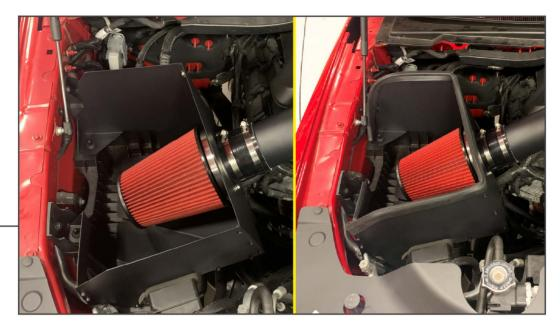
Install the weatherstripping onto the heat shield assembly.
