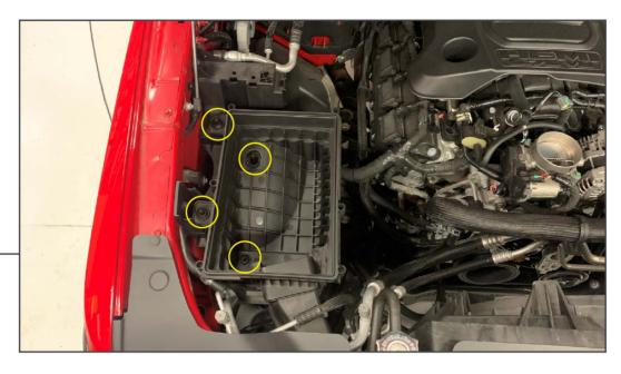
Firmly pull up on the lower air box to dislodge the air box from the mounting pegs in the vehicle.
