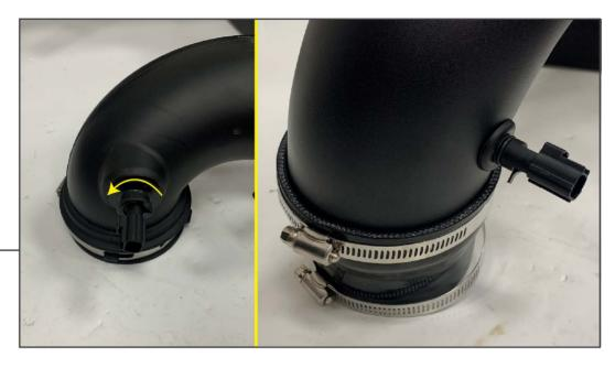
Transfer the intake air temperature sensor from the original intake tube to the new intake tube. Twist the sensor counter-clockwise to remove from the original intake tube. Install the provided (1) rubber grommet into the hole in the intake tube, then push the sensor into the grommet.
