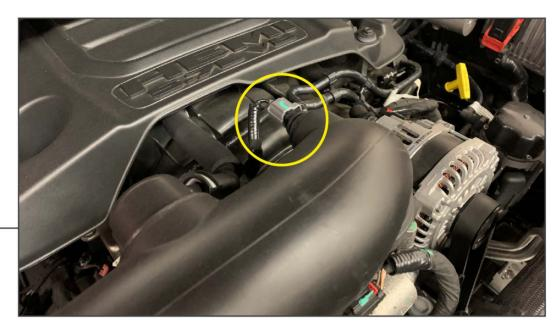
Unplug the intake air temperature sensor from the intake tube.
