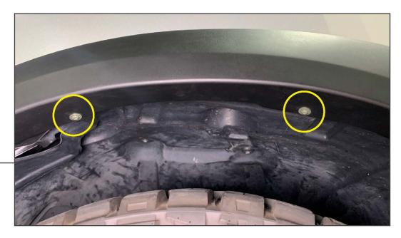
Align the fender flare to the vehicle, then install (2) Phillips screws through the fender flare into the previously installed screw clips. Do not tighten screws.
