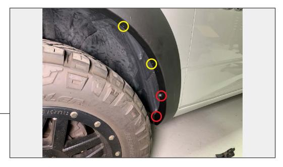
Install (2) Phillips screws and (2) original 10mm bolts into the original fender liner screw clips. Do not tighten screws.
