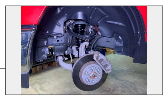
Re-assemble the vehicle suspension following steps 1-8 in reverse order using original hardware. See last page for torque specifications.
