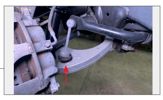
Remove (1) 18mm nut from the bottom of the sway bar link.
