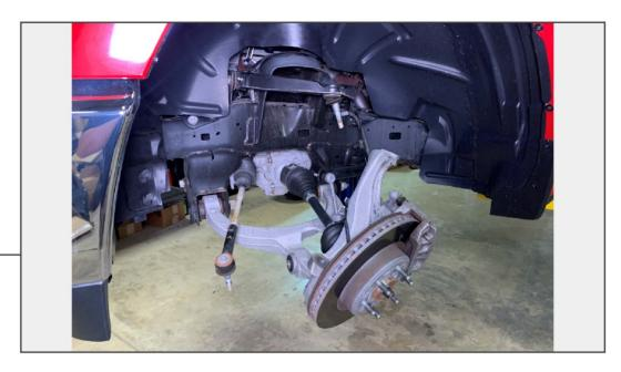
Remove the vehicle strut assembly from the vehicle. Prying downward on the lower control arm with a pry bar may be necessary to gain additional clearance.
