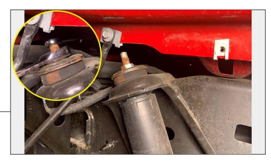
Apply light pressure under the rear axle using a floor jack. Remove (1) 18mm nut from the top of the shock absorber.
