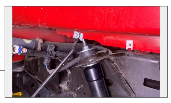
Install the new shock absorber to the vehicle frame using provided hardware. Ensure (1) rubber bushing is on each side of the frame.
