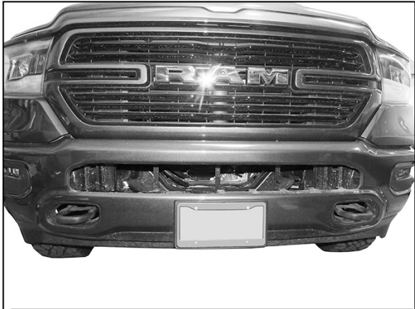
(Fig 2) Center panel removed. Models with sensors, unplug sensors to remove panel
