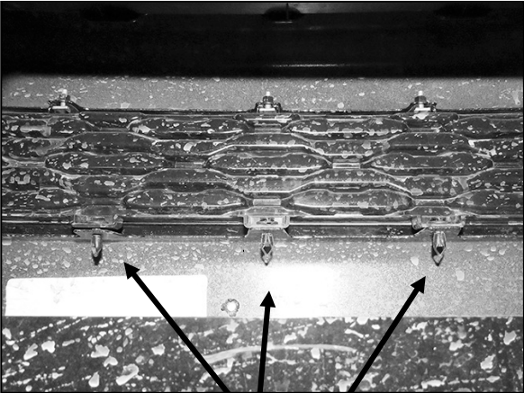
(Fig 1) Release the clips attaching the center plastic panel to the back of the outer bumper cover. NOTE: Panel pictured from behind bumper
