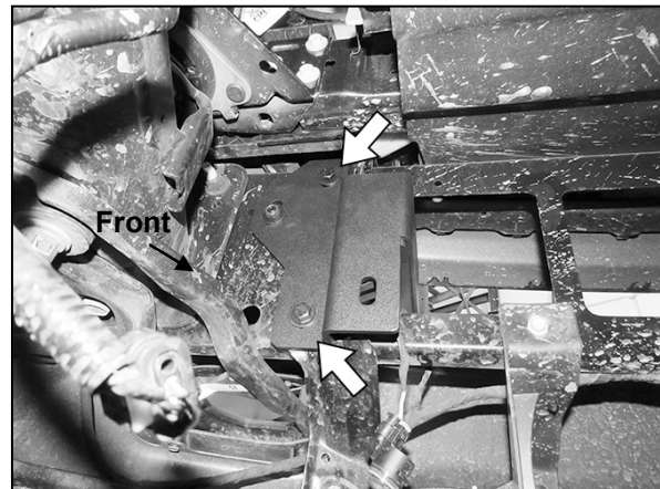
(Fig 8) Driver/left Frame Bracket attached to threaded holes in back of factory bumper bracket (arrows)
