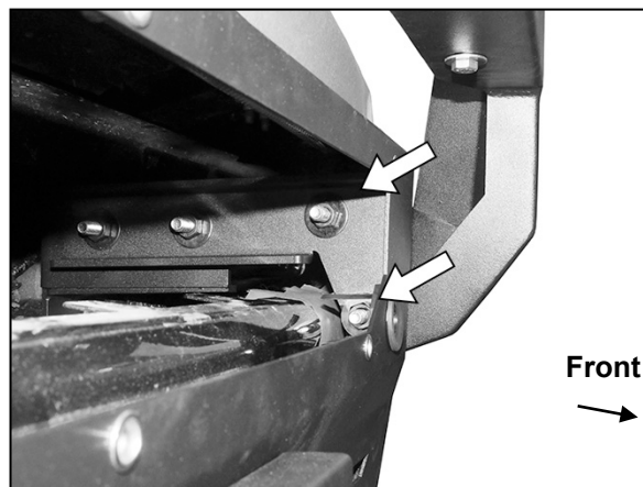
(Fig 23) Driver/left side of Bumper attached to Bracket and Double Bolt Plate (arrows)
