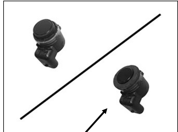
(Fig 25) Remove silicone seal from sensor. Slide large Seal over end of sensor (arrow)
