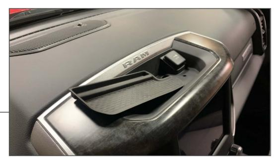
Using a soft pry tool, remove the rubber liner from the dash storage tray. Using a Phillips head screw driver, remove the (2) screws.
