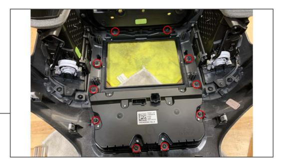
Remove the (10) T-15 Torx screws and remove the HVAC panel from the dash panel.
