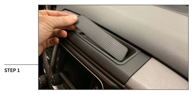
Lift and remove the rubber mat from the storage tray above the radio.
