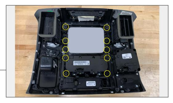
Remove (10) Phillips head screws from the backside of the original radio trim bezel. Remove the A/C control module from the radio trim bezel.
