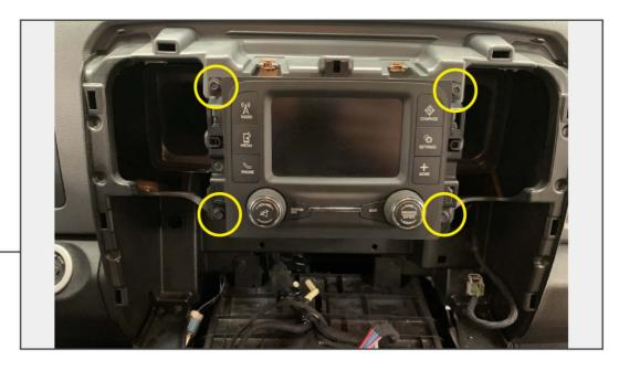
Remove (4) 9/32" screws from the original radio assembly.
