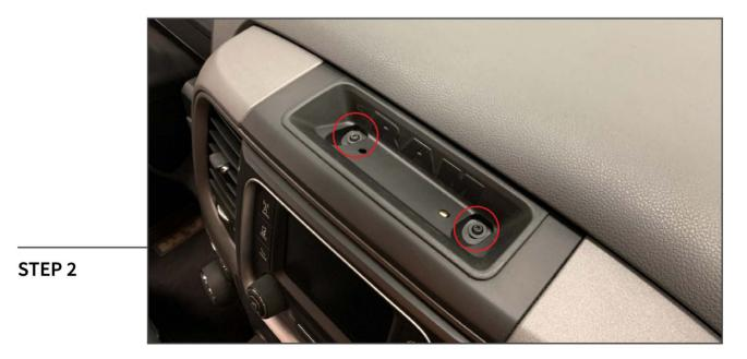
Remove (2) T-20 Torx screws from the top of the dashboard radio bezel.
