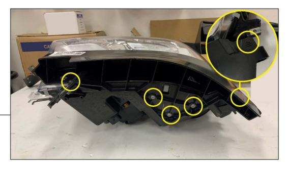
Remove (5) T-25 Torx screws from the lower plastic panel on the headlight. Remove the plastic panel from the headlight. Transfer the plastic panel and hardware to the new LED headlight.
