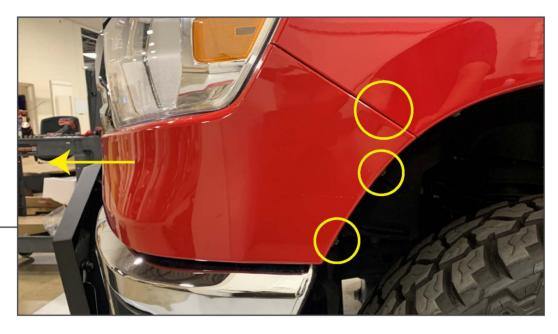
Remove (2) 8mm screws from the inner fender above the front bumper. Remove (1) 10mm bolt connecting the plastic panel to the fender. Peel the plastic panel outward from the fender, then gently pry the front of the panel away from the vehicle.
