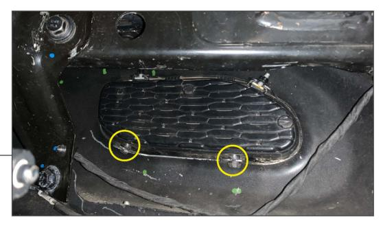
Using a panel removal tool, dislodge the (2) block off plate mounting tabs from the bumper.
