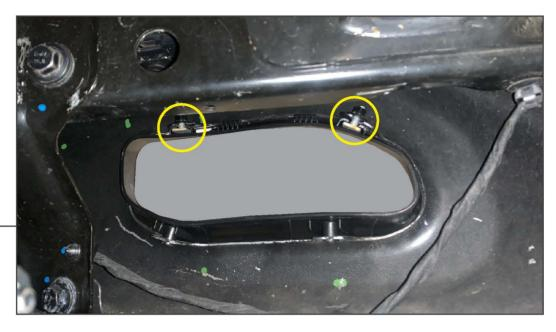
Insert the designated bumper trim panel through the front of the bumper, and secure using the original (2) studs and (2) 10mm nuts.
