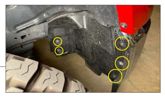
Remove (5) 8mm bolts from the splash guard. Remove the splash guard from the vehicle.
