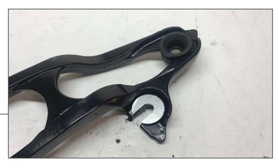
Install (1) bushing into the tow hook. Align (1) 'U' washer to the tow hook.
