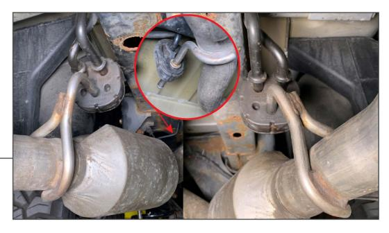
Remove the LH and RH exhaust tail pipes from the rubber exhaust hangers. Remove the tail pipes from the muffler and remove from the vehicle.
