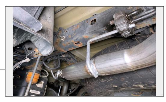
Install the LH rear pipe to the previously installed LH front pipe. Ensure the pipe is in the corresponding rubber exhaust hangers attached to the vehicle. Loosely secure into place using (1) 2.5" exhaust clamp.
