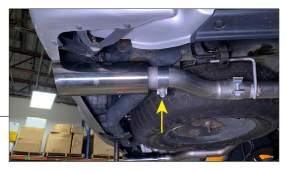
Install (1) exhaust tip to each side of the vehicle exhaust. Loosely secure into place using the welded on exhaust clamp.
