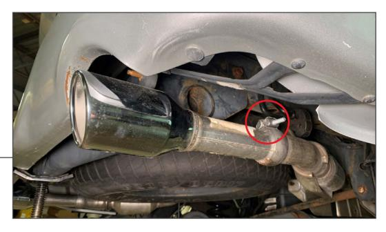
Loosen (1) exhaust clamp at each rear exhaust tip. Remove the exhaust tips from the vehicle.
