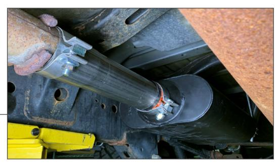
Install the muffler to the previously installed front pipe. Loosely secure into place using (1) 3" exhaust clamp.
