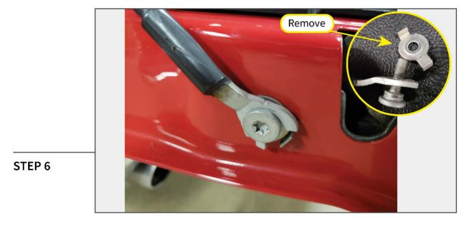
Loosen the lower cable mount. Remove the limiting washer as pictured.
