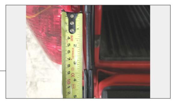
Install the cable clamp 3.5" below the upper cable end. This will prevent the cable from causing damage to the shock.
