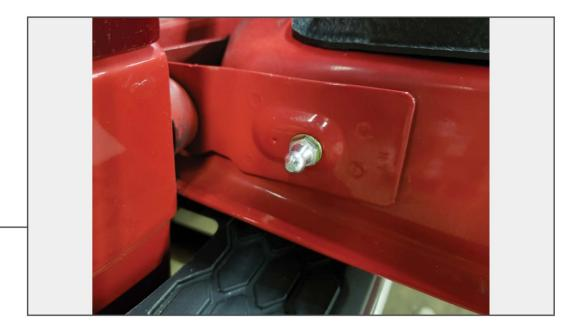
Apply blue thread lock to the threads of the ball mount. Torque the ball mount to 8ft-lbs.
