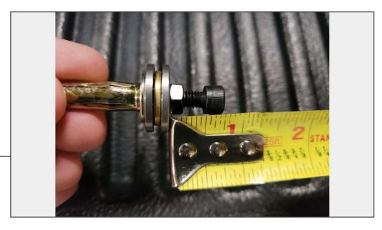
Assemble the nutsert tool as follows: nutsert, washer, bearing, washer, nut, Allen bolt. Adjust the tool so that there is 3/4" between the flat washer and the head of the Allen bolt.
