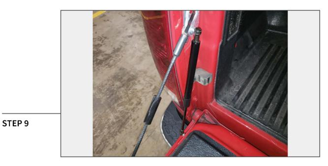
Press the shock onto the ball stud mounts.
