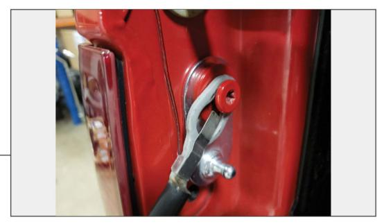
Install the upper ball mount plate behind the upper lift gate Torx bolt. Reinstall lift gate strap.
