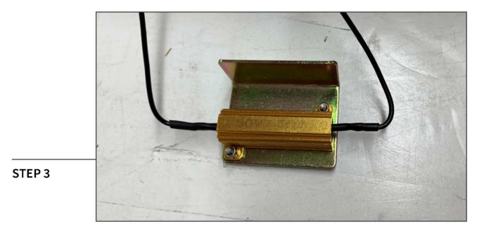
Mount the resistors to the resistor brackets using the supplied hardware. Hold the M4 nut with an adjustable wrench/pliers while tightening the bolts using a Phillips head screwdriver.
