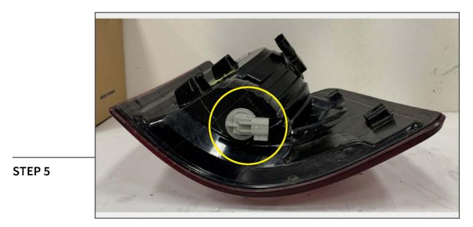
Twist the reverse light bulb socket counter clockwise to remove the socket from the original tail light lens. Install the bulb socket into the new tail light.
