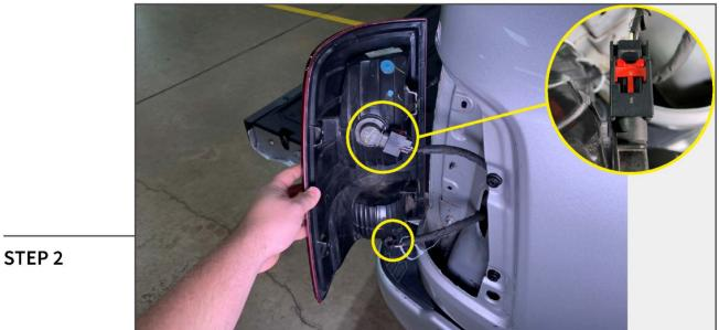
Firmly pull the tail light towards the rear of the vehicle to dislodge the (2) retaining pins. Unplug (2) electrical connectors from the tail light by depressing the plastic tab. Remove the tail light from the vehicle.
