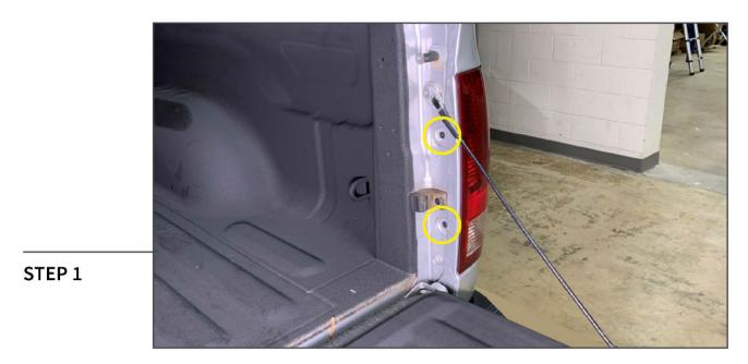
Lower the vehicle tailgate. Remove (2) Phillips head screws from the side of the tail light assembly.
