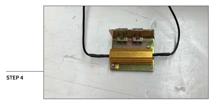
Using (2) vampire clips per bracket, clip each resistor bracket to the vehicle.
