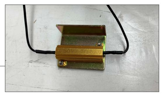
Mount the resistors to the resistor brackets using the supplied hardware. Hold the M4 nut with an adjustable wrench/pliers while tightening the bolts using a Phillips head screwdriver.
