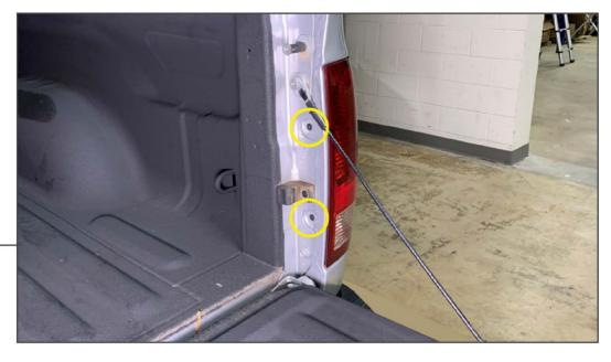
Lower the vehicle tailgate. Remove (2) Phillips head screws from the side of the tail light assembly.
