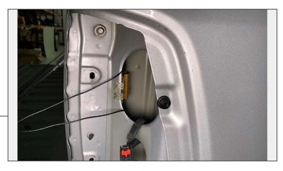
Secure the resistor bracket to the vehicle using the (2) vampire clips.
