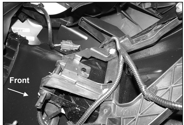
(Fig 2) Unplug fog lights if equipped. Unplug harness to bumper and move harness
