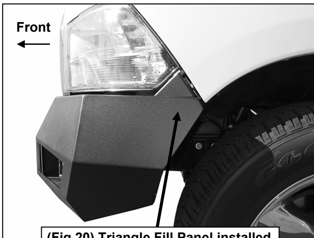
(Fig 20) Triangle Fill Panel installed
