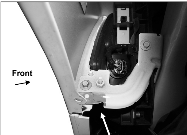
(Fig 3) Pull back fender liner to locate fascia attachment at bottom of front fender
