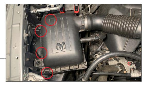
Release the (4) metal clips securing the air box lid to the air box.
