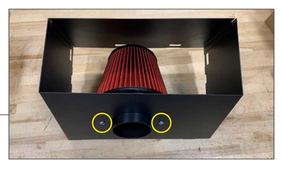
Install the air filter into the heat shield using (2) Allen bolts. Tighten until secure.
