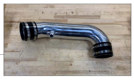
Install the (2) intake tube couplers to the intake tube using (2) large hose clamps. Install the intake tube to the air filter and the throttle body using (2) large hose clamps. Tighten until secure.
