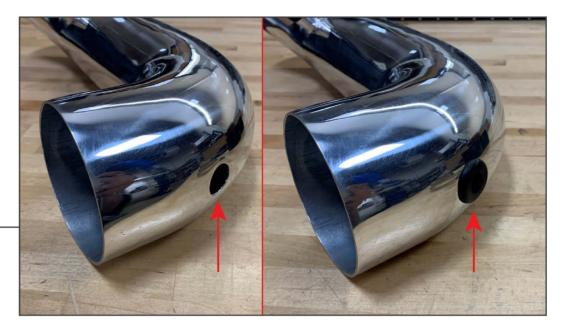
Install the IAT sensor grommet into the intake tube. Spray lubricant may be necessary.
