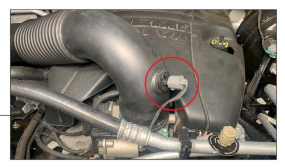
Open the hood of the vehicle. Unplug the IAT sensor connector from the sensor. Twist the sensor counter-clockwise and remove the sensor from the intake tube.
