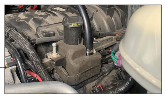
Install the provided PCV hose to the vehicle PCV fitting, secure in place using (1) small hose clamp. Re-install the engine cover to the vehicle.
