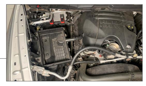
Lift the air box lid and intake tube from the vehicle as an assembly.
