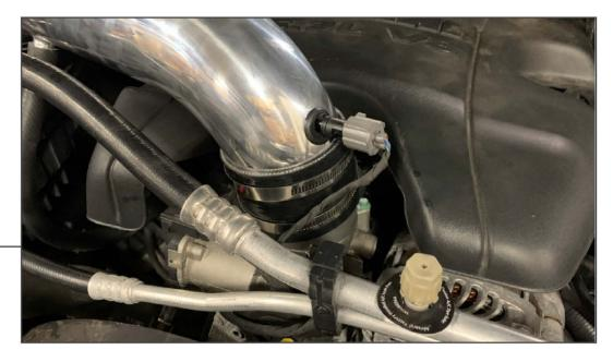
Plug the IAT sensor connector into the IAT sensor. Ensure the connector clicks into place to ensure proper electrical connection.
