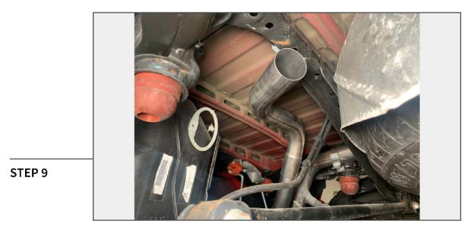
Place (1) 2.5" exhaust clamp onto the LH exhaust pipe, and insert the pipe into the muffler assembly.
