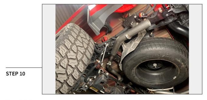
Place (1) 2.5" exhaust clamp onto the LH tail pipe, and insert the pipe into the LH exhaust previously installed.
