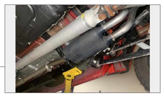
Install the muffler assembly into the (3) rubber hangers. Secure the muffler assembly to the front muffler flange using the (2) original bolts. Re-install ground strap. Fully tighten the flange bolts to 37 ft.-lbs.
