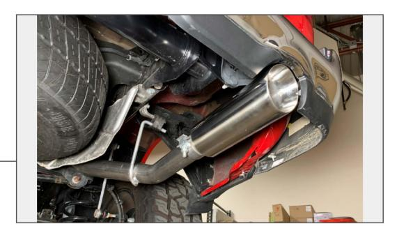
Install the exhaust tips onto the LH and RH tail pipes to determine final install location. Adjust the pipes to the appropriate exhaust fitment.
