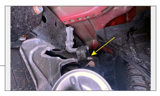
Use spray lubricant on the rear muffler exhaust hangers. Remove the RH side muffler pipe first, and remove the pipe assembly from the vehicle. Remove the LH side muffler hanger from the rubber hanger.
