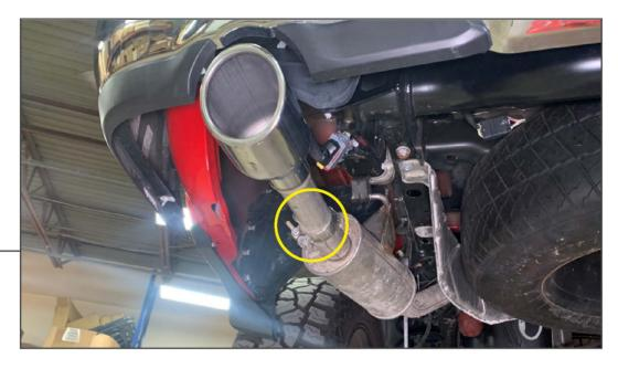
Lift and support the vehicle using a jack and jack stands. Loosen (1) exhaust clamp and remove the exhaust tip from the vehicle exhaust.
