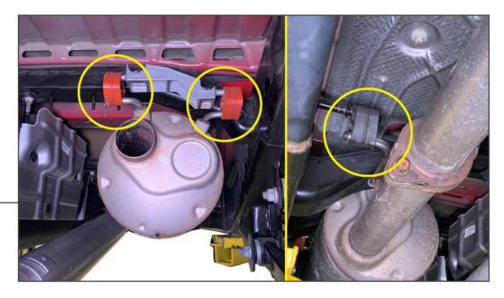
Disconnect the (2) exhaust hangers from the top of the muffler assembly, following with the (1) exhaust hanger at the front muffler flange. Remove the ground strap, then remove the exhaust system from the vehicle.
