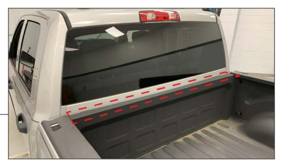
Clean the bulkhead area of the vehicle bed using isopropyl alcohol and a microfiber cloth. Once dry, adhere the bulkhead gasket to the bulkhead, trim to size as necessary.
