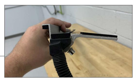
At the opposite side of the side rail, insert (1) tonneau retaining bracket. Do not tighten the Allen bolt. Install (1) drain tube end cap onto the side rail.
