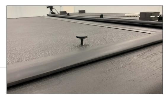
Unfold the first panel of the tonneau cover. Locate (1) hole on each side of the first tonneau cover panel. Align the tonneau mounting brackets on the side rails to the holes. Insert (1) stud and (1) rubber flat washer through the tonneau cover on each side.
