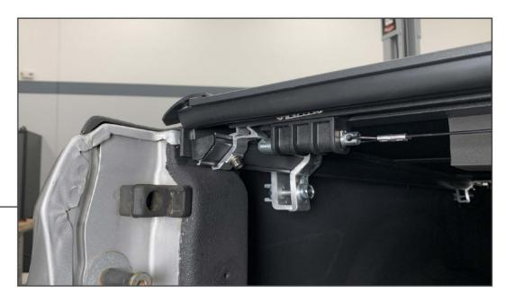
Adjust the locking brackets to the tonneau cover latches. Ensure the latches and the bracket are properly aligned for proper functionality. Once adjusted, tighten the Allen bolt on the locking bracket.
