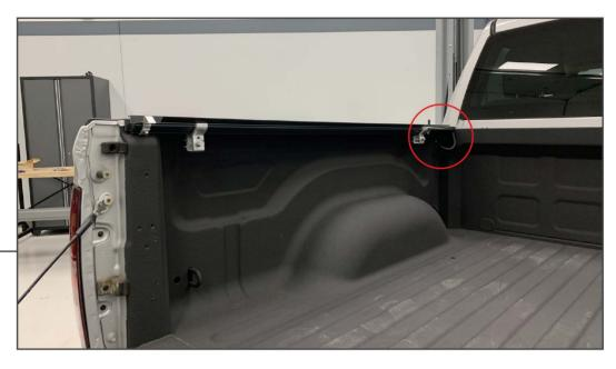
Insert the drain tube on the side rail into the hole in the vehicle bed. Ensure the tube is routed towards the outside of the vehicle.
