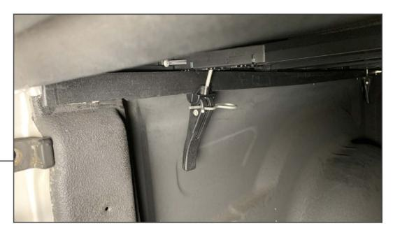
Unfold the tonneau cover towards the rear of the vehicle. Secure the (2) pre-installed rear clamps to the metal portion of the vehicle bed rails. Lock the clamps into place using (1) cotter pin per clamp.
