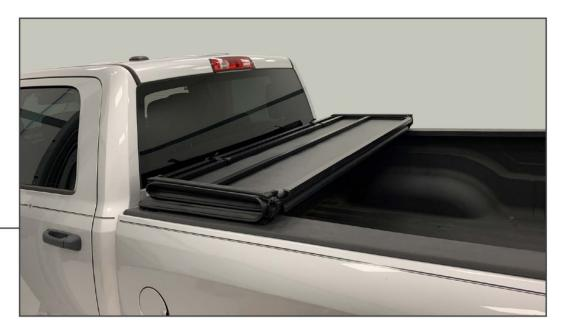
Place the tonneau cover onto the vehicle bed closest to the cab. Ensure the panel with the yellow safety straps are facing downwards towards the bed floor.
