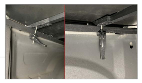
Once aligned, carefully fold the tonneau cover up towards the cab of the vehicle to access the (2) pre-installed front clamps. Tighten the clamps upwards, then hook the clamp onto the metal portion of the bed rail. Fold the clamp handle 90 degrees to add tension to secure the cover.
