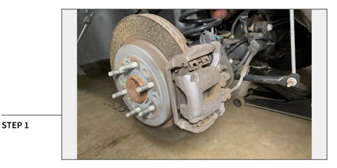
Lift and support the vehicle using a floor jack and jack stands. Remove the wheel from the vehicle to expose the brake caliper.
