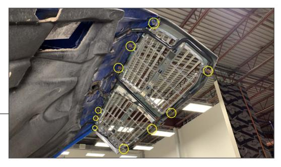
Open the vehicle hood. Remove (10) 8mm screws from the grille attached to the vehicle hood.
