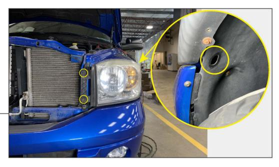
Remove the LH front headlight by removing (2) 10mm bolts from the front of the vehicle. Remove (1) 10mm bolt by the access hole in the fender liner.
