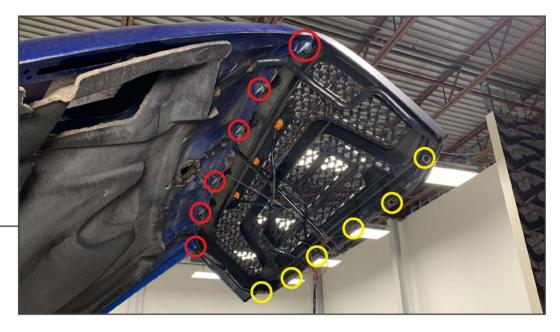
Align the new grille and secure the top using (6) flat washers and (6) lock nuts. Secure the bottom of the grille using the provided (6) screws.
