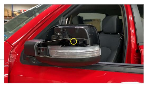
Install the new light into the mirror lower cover using the original hardware. Plug the wiring harness into the vehicle harness, ensuring to enable the locking tab. Install the lower cover to the mirror assembly, ensuring the wiring harnesses are neatly routed away from mirror cover mounting points.
