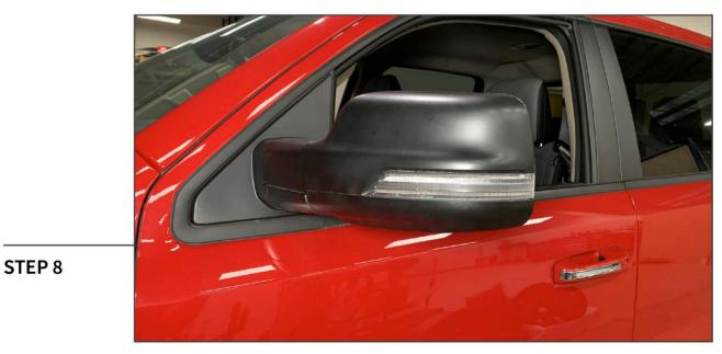
Re-assemble the vehicle mirror following steps 1-4 in reverse order. Ensure the mirror glass is secure on the mount.
