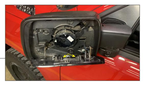
Angle the mirror glass downwards to access the backside of the mirror glass. Using a flathead screwdriver, dislodge the (2) mirror glass retainers, while applying pressure to pull the mirror glass away from the vehicle.
