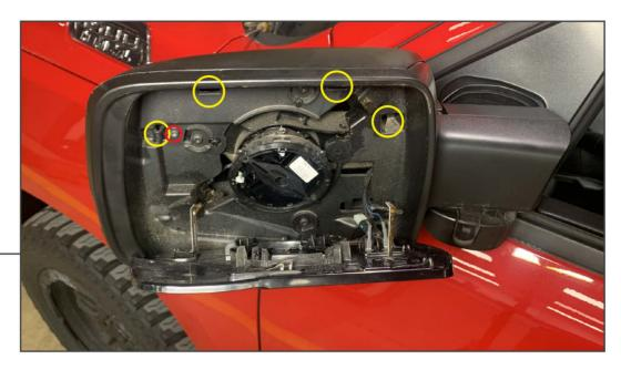
Remove (1) T-20 Torx screw from the exterior upper mirror cover. Using a flathead screwdriver, depress the (4) plastic tabs, and remove the exterior upper mirror cover from the vehicle.
