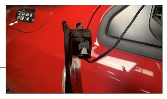
Locate the electrical connector on the mirror light. Slide the gray tab back, and press and remove the connector from the light.
