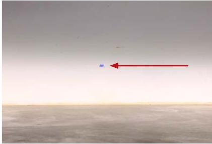
11. Aim your SS3 pods on each side, so that the top of the beam pattern is on the cutoff line mark.
