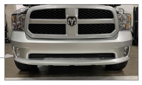
Firmly pull the lower splash guard away from the front bumper assembly.
