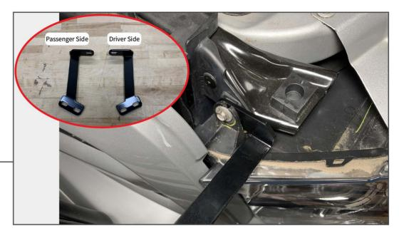
Place the upper mounting bracket between the radiator support and the headlight mounting tab. Secure the bracket into place using the original 10mm bolt. Do not fully tighten.
