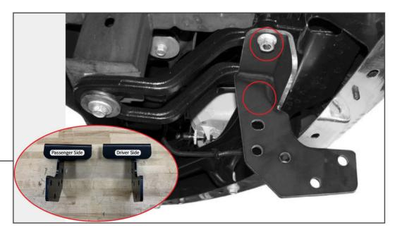
For vehicles with OEM Tow Hooks: Loosely secure the lower mounting bracket to the tow hook studs using the (2) original 18mm nuts.
