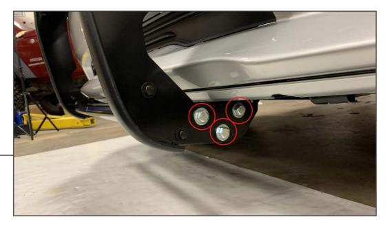
Align the grille guard to the lower mounting brackets, ensuring the brackets are on the inside of the grille guard. Secure the grille guard to the brackets using (3) M12x1.75 x 35mm bolts, (3) M12 lock washers, (6) M12 flat washers, and (3) M12 nuts per side.
