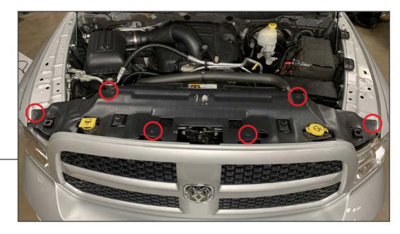
Open the vehicle hood. Remove the upper splash shield by removing (6) plastic push clips.
