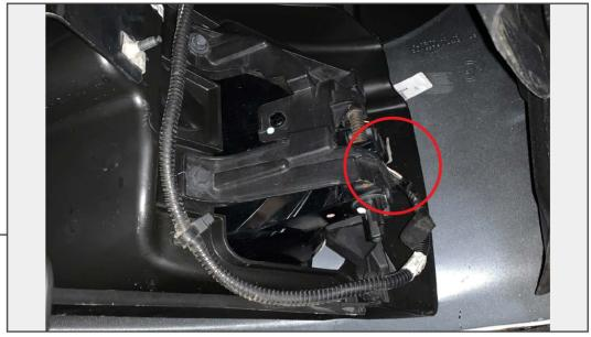
From behind the front bumper, unplug the fog light electrical connector.
