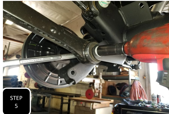
Step 5 Unbolt the trac bar from the mount on the frame and separate. Next, loosen all 8 bolts attaching all 4 control arms just enough to take tension off of the bushings.
