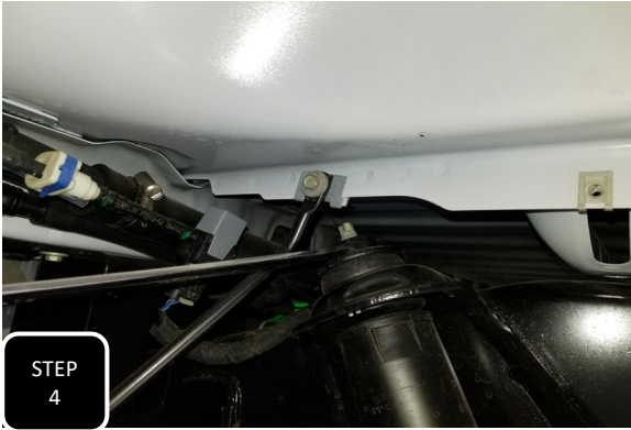
Step 4 Unbolt both rear shocks at both ends and remove them.
