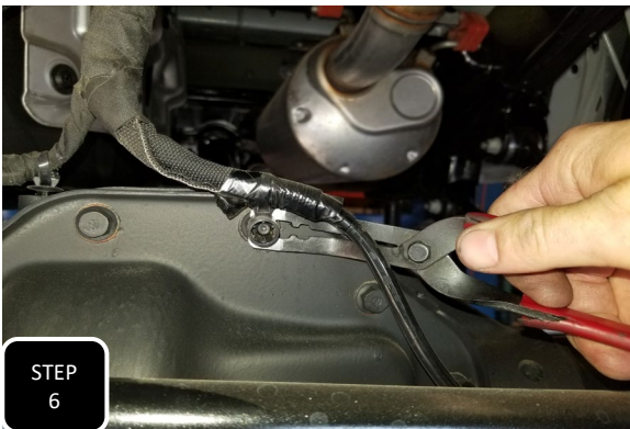
Step 6 Separate the guide clips attaching the ABS lines to the differential in order to gain slack in the line for when the axle gets lowered.
