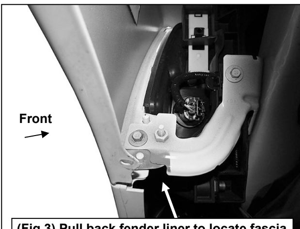
(Fig 3) Pull back fender liner to locate fascia attachment at bottom of front fender
