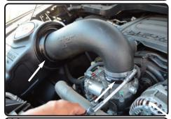
**16.** Once positioned and adjusted properly, tighten all clamps using 8mm nut driver.
