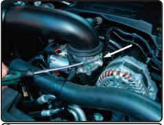
**3.** Loosen the clamp on the throttle body using 8mm nut driver.
