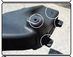
7. Remove the 4 factory grommets from the OEM air box and install to the new air box and secure.
