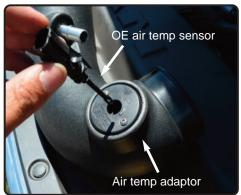
**14.** Install the temperature sensor into the adaptor. twist and lock into place.
