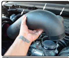
**15.** Install the intake tube and position the intake tube to the filter and the tube to the throttle body.
