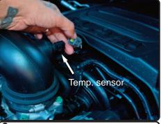
**2.** Disconnect the Temperature sensor harness. Remove the temperature sensor harnes by twisting and pulling out of intake tube.
