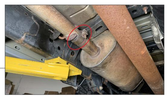
Loosen the (1) exhaust clamp securing the muffler to the vehicle front pipe. Once loose, dislodge the muffler from the (2) rubber hangers and remove the muffer from the vehicle.
