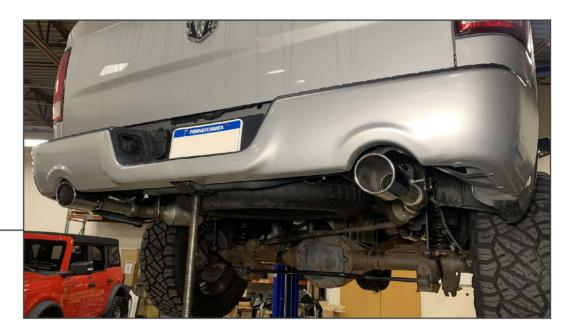
Re-install the original exhaust tips. Adjust the exhaust to allow proper clearance from other components. The 'Y' pipe is designed to have generous inwards/outwards movement for additional tailpipe adjustments. Once adjusted, tighten all exhaust clamps to 45 ft.-lbs.
