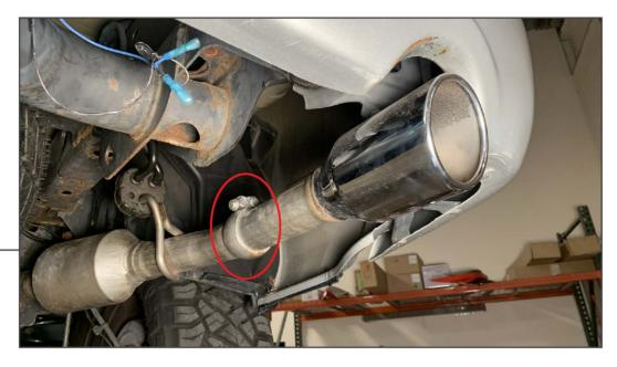
Lift and support the vehicle using a floor jack and jack stands. Remove the exhaust tips from the exhaust system by loosening the (1) exhaust clamp per tip.
