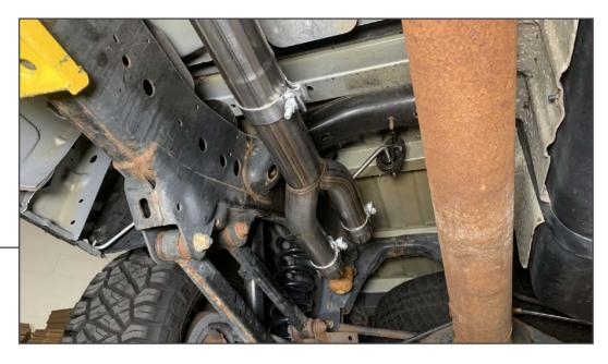
Place the 'Y' pipe hangers into the vehicle rubber hangers, then insert the 'Y' pipe into the previously installed front pipe. Secure the pipes together using the previously placed (1) 3" exhaust clamp.
