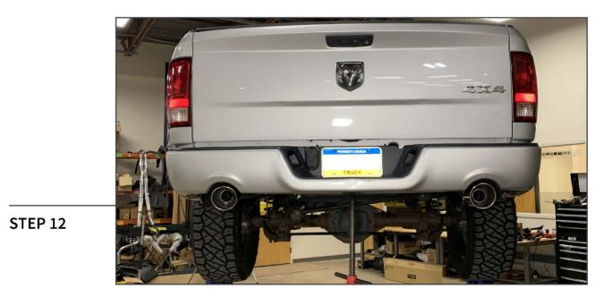
Place the exhaust tip to the tail pipe, and secure using the previously installed ball flange exhaust clamp. Adjust the exhaust as necessary, ensuring proper clearance, then tighten all clamps to 45 ft./lbs. Adjust the exhaust tips to the desired position, and tighten the clamps to 25 ft./lbs.
