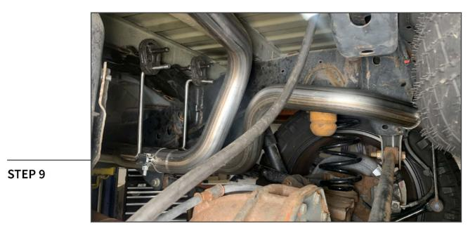
Install the RH over axle pipe pipe into the 'Y' pipe. Loosely secure the pipes using the previously installed clamp.
