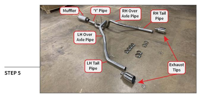
Lay out and identify all exhaust components.
