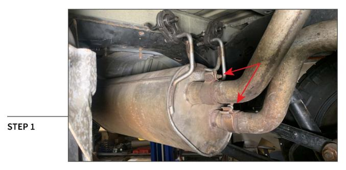
Lift and support the vehicle using a floor jack and jack stands. Loosen the (2) exhaust clamps from the muffler outlet.
