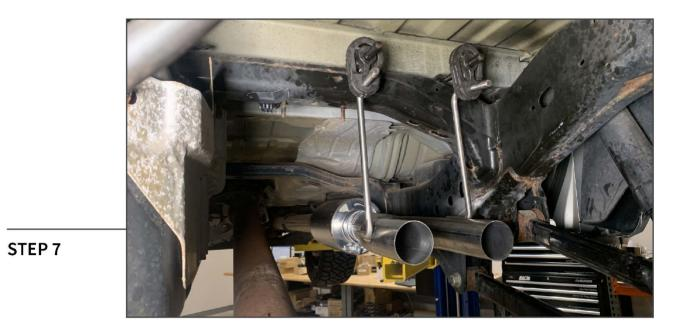
Install the 'Y' pipe into the muffler, and insert the (2) rubber hangers into the body mounting points.
