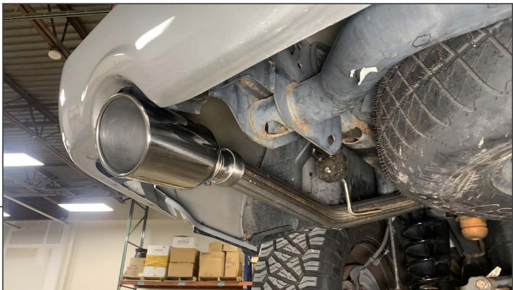
Install the LH tail pipe into the over axle pipe, and insert the (1) rubber hanger into the body mounting points. Loosely secure the pipes using the previously installed clamp.
