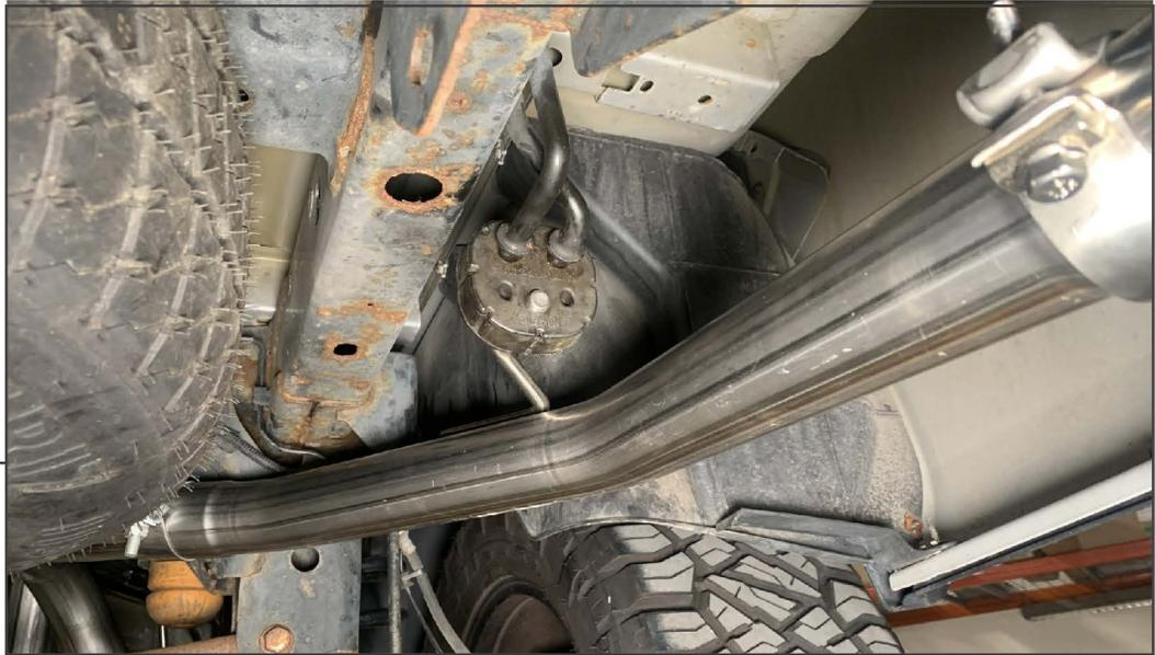
Install the RH tail pipe into the over axle pipe, and insert the (1) rubber hanger into the body mounting points. Loosely secure the pipes using the previously installed clamp.
