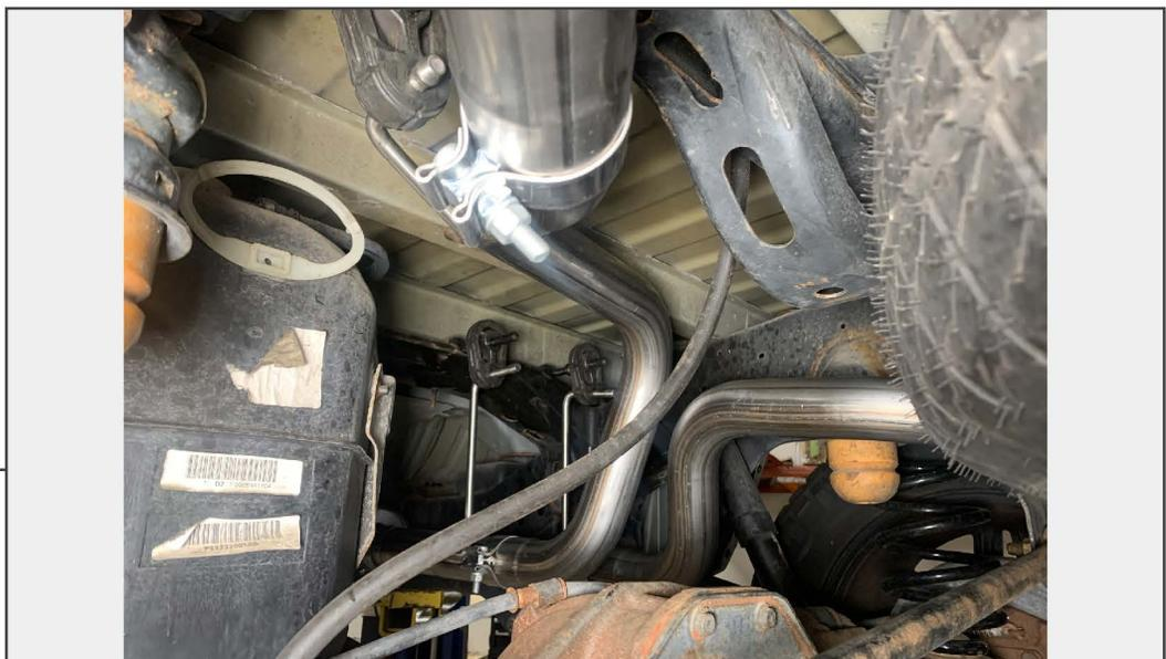
Install the LH over axle pipe into the 'Y' pipe, and insert the (1) rubber hanger into the body mounting points. Loosely secure the pipes using the previously installed clamp.
