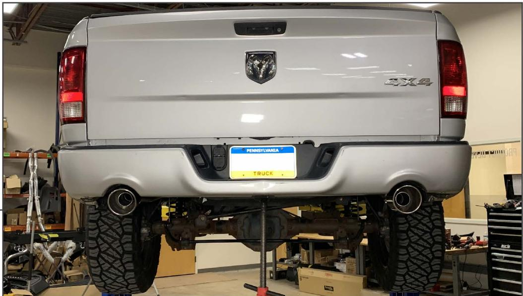
Place the exhaust tip to the tail pipe, and secure using the previously installed ball flange exhaust clamp. Adjust the exhaust as necessary, ensuring proper clearance, then tighten all clamps to 45 ft./lbs. Adjust the exhaust tips to the desired position, and tighten the clamps to 25 ft./lbs.
