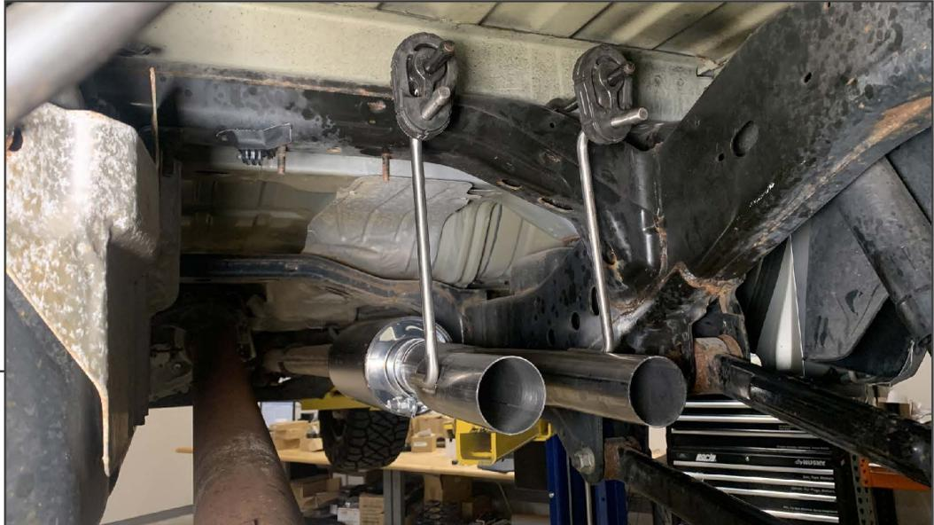
Install the 'Y' pipe into the muffler, and insert the (2) rubber hangers into the body mounting points.
