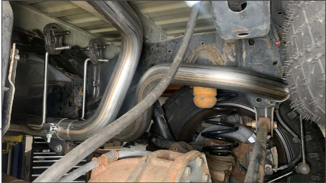
Install the RH over axle pipe pipe into the ‘Y’ pipe. Loosely secure the pipes using the previously installed clamp.
