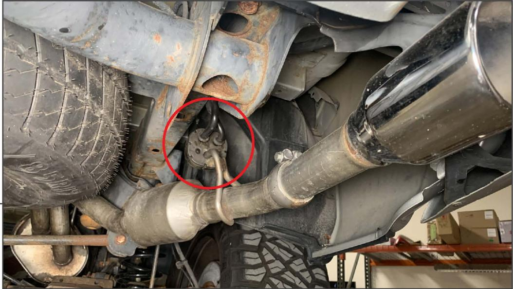
On the RH side of the vehicle, disconnect (1) rubber hanger securing the exhaust pipe to the vehicle. With the hanger disconnected, slide the pipe out from the muffler and set aside.
