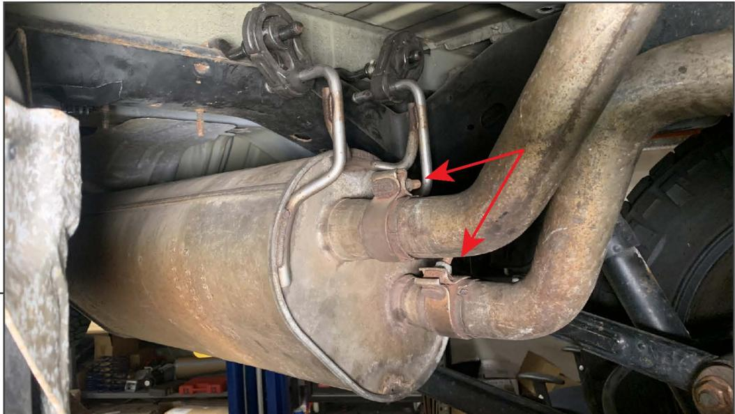
Lift and support the vehicle using a floor jack and jack stands. Loosen the (2) exhaust clamps from the muffer outlet.
