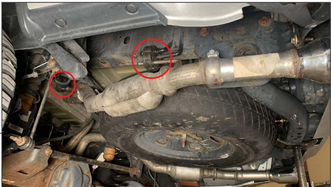
On the LH side of the vehicle, disconnect (2) rubber hangers securing the exhaust pipe to the vehicle. With the hangers disconnected, slide the pipe out from the muffer and set aside.
