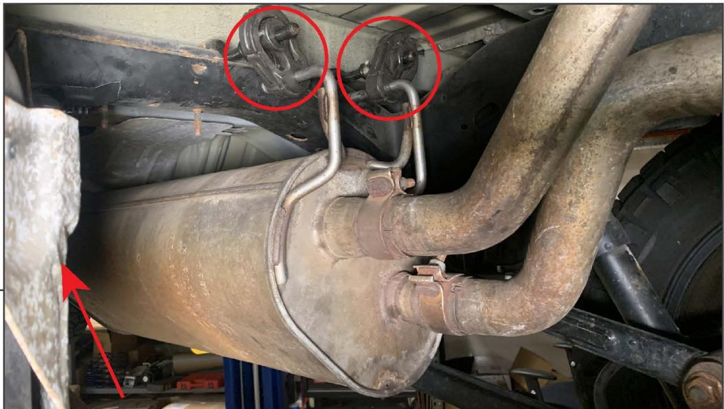
Loosen (1) exhaust clamp at the muffler inlet. Once loose, disconnect (2) rubber hangers securing the muffler to the vehicle. With the hangers disconnected, slide the muffler off of the front pipe and set the muffler aside.
