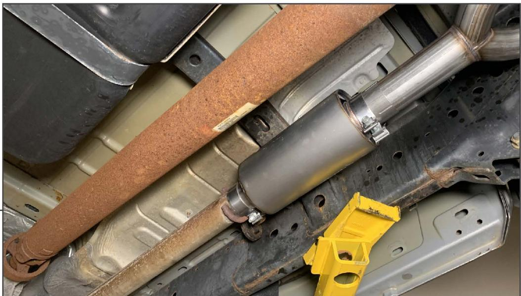
Place (1) 3" exhaust clamp onto the vehicle front pipe, then place the new muffler onto the front pipe. Loosely secure the muffler to the pipe.
