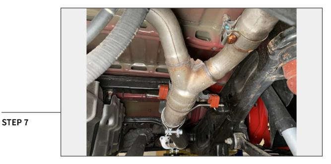
Insert the tailpipe assembly into the 'S' pipe. Install the LH and RH tailpipes and exhaust tips into the vehicle using the original clamps and rubber hangers.
