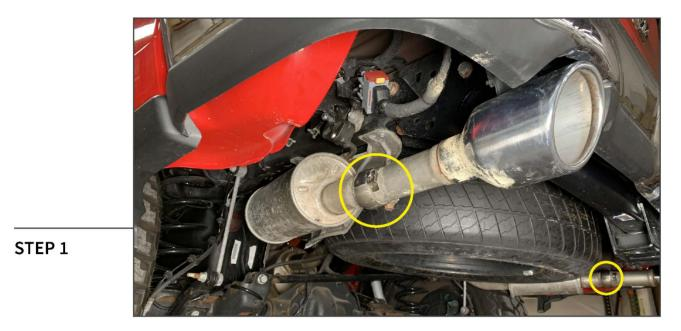
Lift and support the vehicle using a floor jack and jack stands. Locate and remove the (2) exhaust tip pipes from the exhaust by loosening the exhaust clamps.
