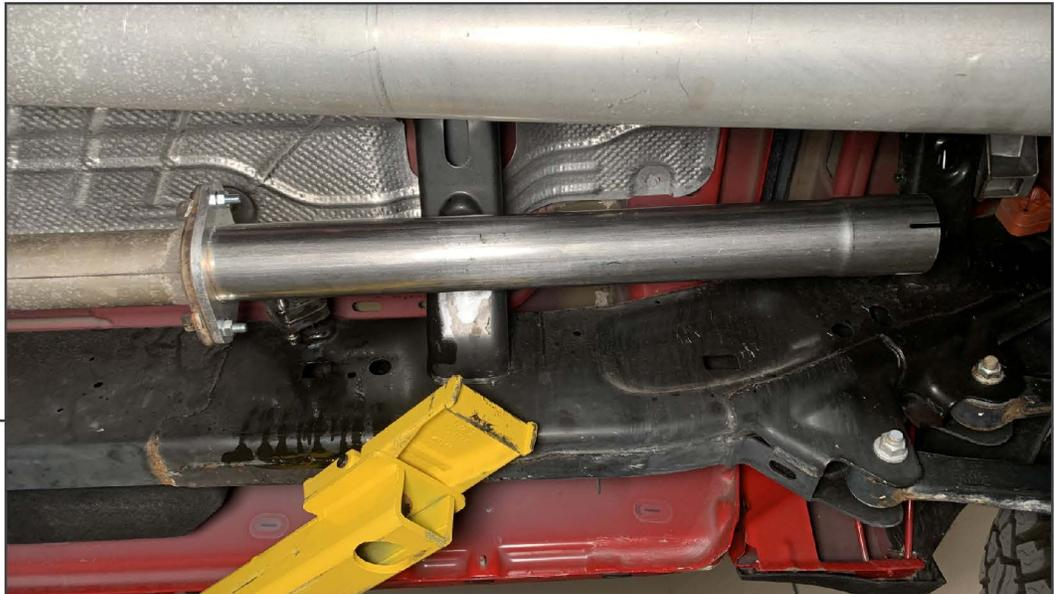
Align the (1) straight pipe to the vehicle exhaust flange, and insert the (1) metal hanger into the vehicle rubber hanger. Thread the included hardware into the flanges, but do not fully tighten to allow for later adjustment.
