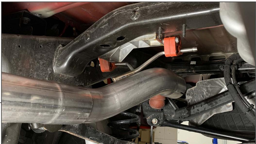
Align the (1) 'S' pipe to the previously installed straight pipe. Insert the (2) metal hangers into the vehicle muffler hangers.
