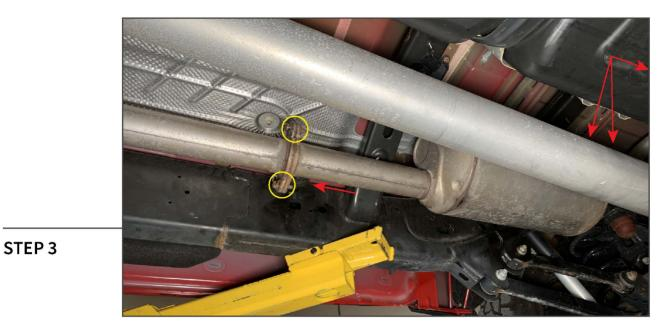
Remove (2) 16mm bolts from the front muffler flange to disconnect the muffler from the front portion of the vehicle exhaust. Disconnect the (3) muffler rubber hangers, and (1) LH tailpipe rubber hanger, then remove the exhaust assembly from the vehicle.
