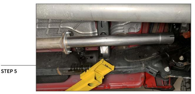
Align the (1) straight pipe to the vehicle exhaust flange, and insert the (1) metal hanger into the vehicle rubber hanger. Thread the included hardware into the flanges, but do not fully tighten to allow for later adjustment.
