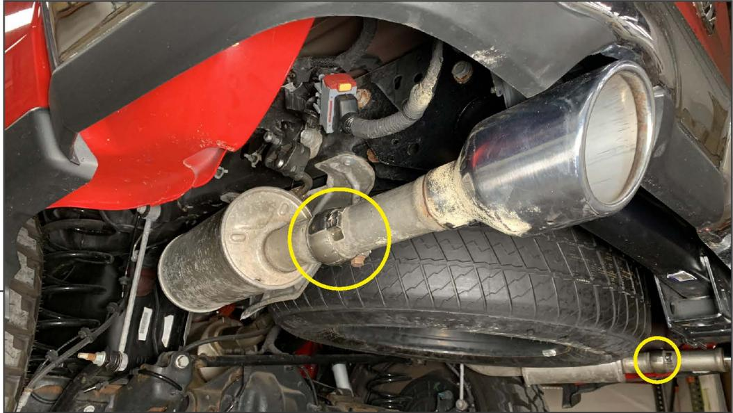
Lift and support the vehicle using a floor jack and jack stands. Locate and remove the (2) exhaust tip pipes from the exhaust by loosening the exhaust clamps.
