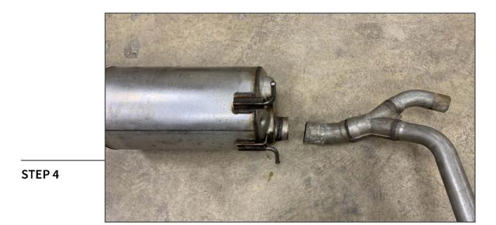
Place the muffler on a workable surface for cutting. Mark the muffler 2-3" from the end of the outlet port. Once marked, cut the tailpipe assembly from the muffler using a saw.
