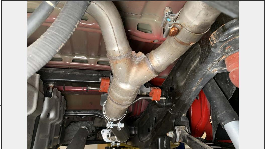
Insert the tailpipe assembly into the 'S' pipe. Install the LH and RH tailpipes and exhaust tips into the vehicle using the original clamps and rubber hangers.
