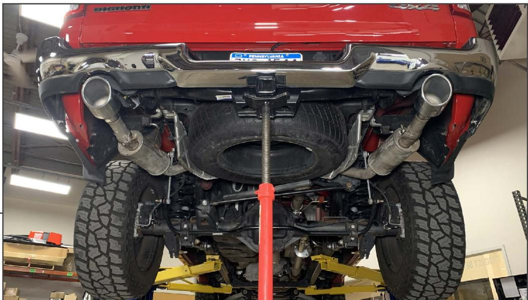
Adjust the exhaust as necessary for best fit. Tighten the exhaust down using the following torque specifications. Installation is now complete.
