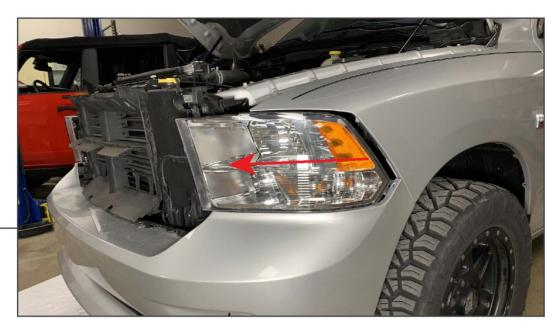
Pull the headlight away from the vehicle to dislodge the (1) alignment dowel.
