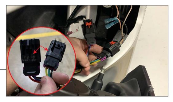
Plug the adapter harness into the new headlight. Then, plug the (2) adapter harness connectors into the vehicle wiring harness.
