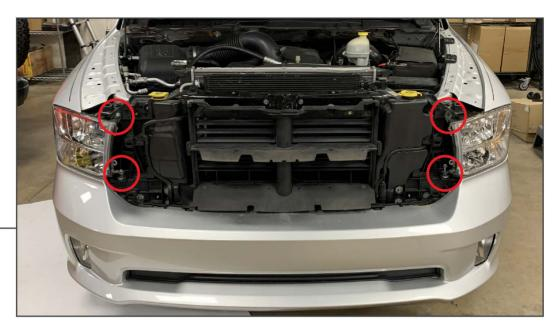
Remove (2) 10mm bolts from each headlight assembly.
