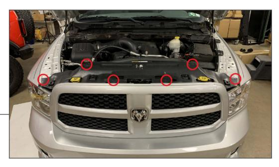
Open the vehicle hood. Remove (6) plastic push clips from the upper radiator cover. Remove the cover and set aside.
