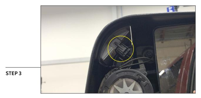
Unplug the electrical connector from the mirror turn signal light housing.
