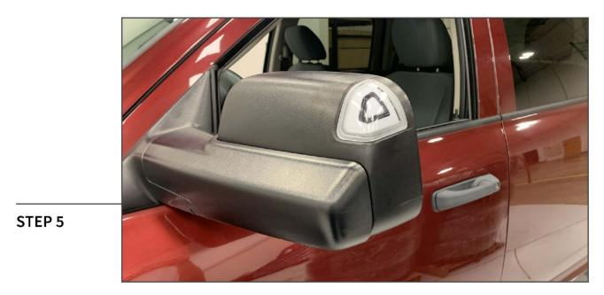
Fit the new mirror turn signal lamp into the mirror, and ensure the lamp is properly seated. Secure the lamp into place reusing the original (1) T-15 Torx screw.
