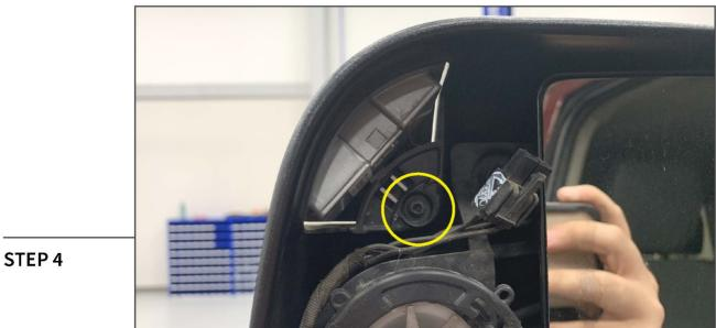
Remove (1) T-15 Torx screw from the turn signal light housing. Remove the vehicle turn signal light from the vehicle mirror.
