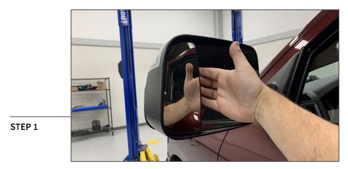
Adjust the mirrors to allow your hand to fit behind the small mirror glass.
