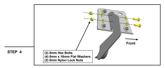
Loosely connect the (1) Driver Front step bracket to the (1) Driver Front reinforcement bracket using (2) M8 x 25mm hex bolts, (4) M8 x 16mm flat washers, and (2) M8 nylon lock nuts.
