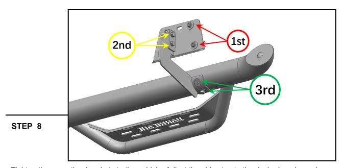
Tighten the mounting brackets to the vehicle. Adjust the side step to the desired angle, and tighten the M8 combo bolts to secure the step into place. See photo for tightening order visual.
