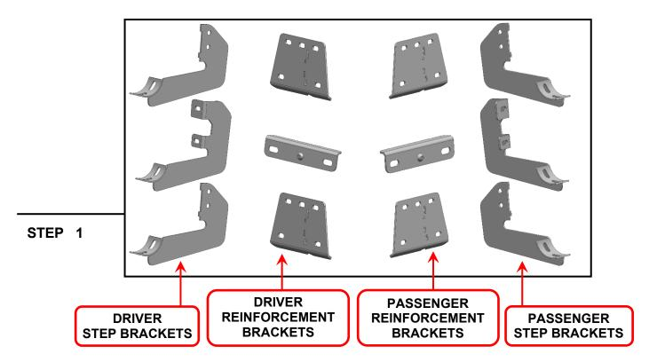
Identify each mounting bracket using the engraved location identifier. Notice: The 4 sets Front and Rear step brackets & reinforcement brackets are the same. The 2 sets Center step brackets & reinforcement brackets are the same.
