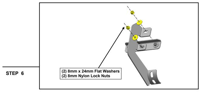
Loosely connect the (1) Driver Center step bracket to the (1) Driver Center reinforcement bracket using (2)  $M8 \times 24$ mm flat washers, and (2) M8 nylon lock nut.
