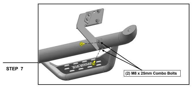
With all brackets loosely mounted to the vehicle, fit the side step onto the brackets, and loosely secure into place using (6) M8 x 25mm combo bolts.
