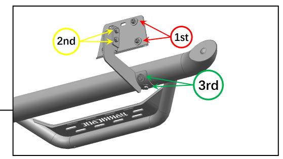
Tighten the mounting brackets to the vehicle. Adjust the side step to the desired angle, and tighten the M8 combo bolts to secure the step into place. See photo for tightening order visual.
