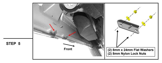
Loosely fit the (1) Driver Center reinforcement bracket to the (2) lower threaded studs using (2) M8 x 24mm flat washers, and (2) M8 nylon lock nuts. Do not fully tighten to allow for later adjustments.
