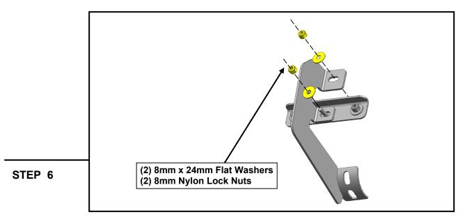
Loosely connect the (1) Driver Center step bracket to the (1) Driver Center reinforcement bracket using (2) M8 x 24mm flat washers, and (2) M8 nylon lock nut.
