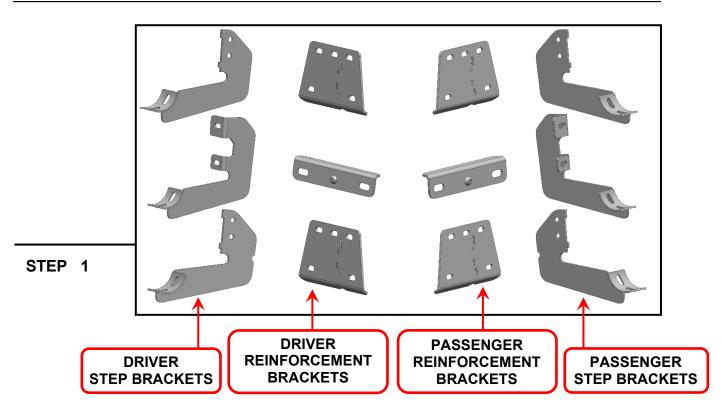
Identify each mounting bracket using the engraved location identifier. Notice: The Front reinforcement brackets and the Rear reinforcement brackets are the same. The Rear step brackets different from the Front step brackets - a notch is cut in the rear of the Rear step bracket.
