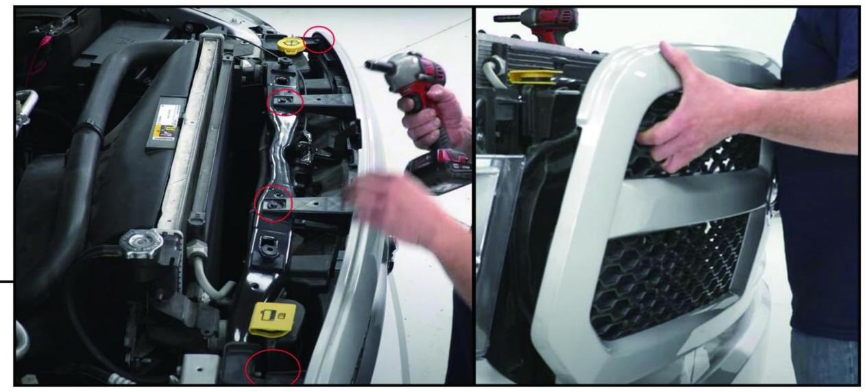
Use tools to remove the bolts and remove the cover panel.
