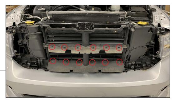
Remove the air dampers from the shutter assembly using a panel removal tool & a Phillips screw-driver.
