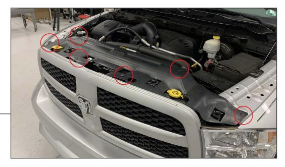
Remove (6) plastic push clips from the upper radiator cover. Then, remove the cover from the vehicle and set aside.
