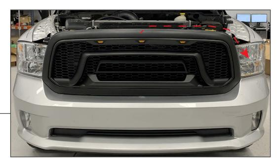
Neatly route the wiring harness towards the Driver's Side headlight assembly. Splice the LED DRL lights into the vehicle parking lamps following the diagram below using the (2) scotchlok connectors. Ensure to route the harness away from hot/moving components.
