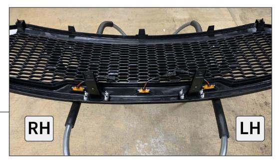
Identify the included mounting brackets using the "L" and "R" identification markings. "L" is to fit to the Driver's Side of the vehicle, while "R" is for the Passenger's Side of the grille.
