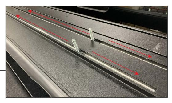
Fit the head of (4) M8 bolts into the front of the tonneau cover. Slide (2) bolts to the driver's side and (2) bolts to the passenger's side.
