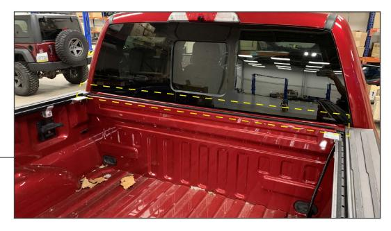
Clean the vehicle bulkhead using isopropyl alcohol and a microfiber cloth, allow to dry. Then, adhere the bulkhead gasket to the vehicle bulkhead.
