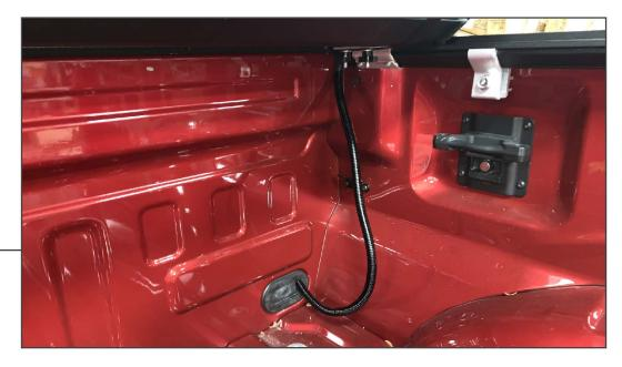
Fit (1) drain tube into the side rail fitting. Route the drain tube towards the vehicle bed grommet. Carefully cut a slot in the grommet to route the drain, or remove the grommet from the bed.
