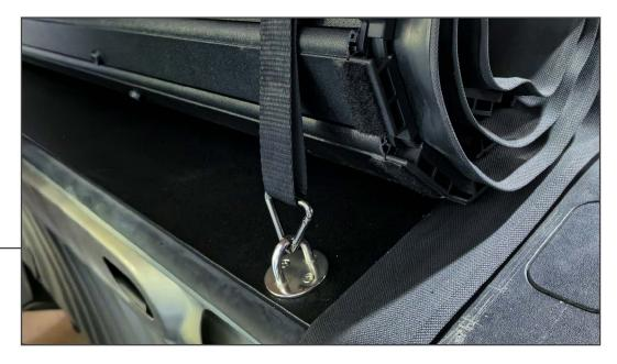
To store the tonneau cover, roll the tonneau cover towards the vehicle cab, and secure each side using the straps into the retainers in the tonneau cover panel. Ensure the straps are tightened after clipping into place.
