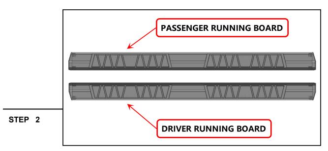
Identify each side step by the front of the step. Notice: "D" for Driver/Left Side; "P" for Passenger/Right Side.
