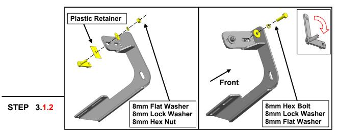
Loosely connect the (1) Driver Front step bracket to the threaded end of the Bolt Plate using (1) Plastic Retainer, (1) M8 hex nut, (1) M8 x 24mm flat washer, and (1) M8 lock washer.
