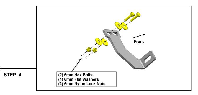
Loosely connect the (1) Driver Front reinforcement bracket to the back of the pinch weld using (2) M6  $\times$  25mm hex bolts, (2) M6  $\times$  22mm flat washers, and (2) M6 nylon lock nuts.
