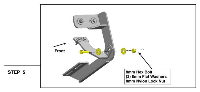
Loosely connect the (1) Driver Front step bracket to the (1) Driver Front reinforcement bracket using (1) M8 × 25mm hex bolt, (2) M8 × 24mm flat washers, and (1) M8 nylon lock nut.
