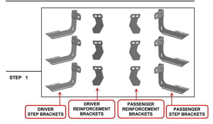
Please identify each mounting bracket using the engraved location identifier. Notice: The step brackets & reinforcement brackets per side are the same.
