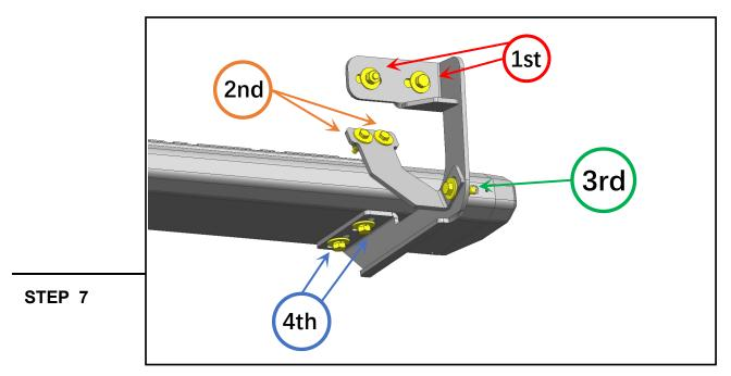
Tighten the mounting brackets to the vehicle. Adjust the Running Board to the desired angle, and tighten the M8 combo bolts to secure the step into place. See photo for tightening order visual.
