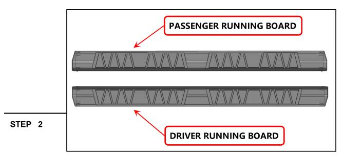
Identify each side step by the front of the step. Notice: "D" for Driver/Left Side; "P" for Passenger/Right Side.
