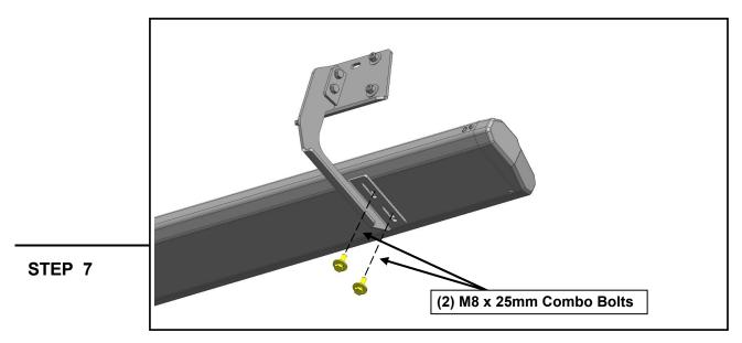
With all brackets loosely mounted to the vehicle, fit the Driver/Left Running Board onto the brackets, and loosely secure into place using (6) M8 x 25mm combo bolts.
