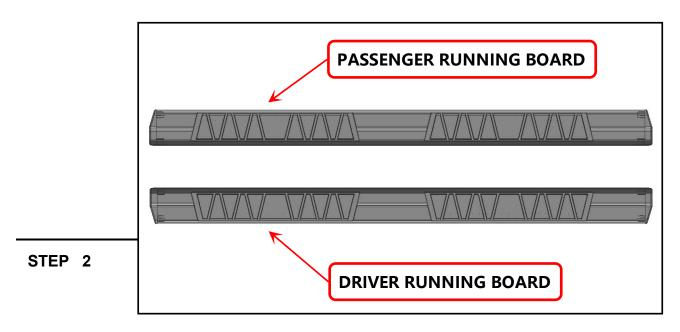
Identify each side step by the front of the step. Notice: "D" for Driver/Left Side; "P" for Passenger/Right Side.
