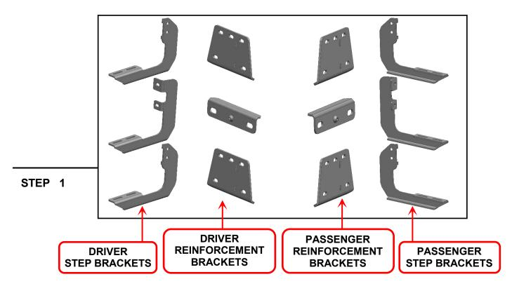
Please identify each mounting bracket using the engraved location identifier. Notice: The 4 sets Front and Rear step brackets & reinforcement brackets are the same. The 2 sets Center step brackets & reinforcement brackets are the same.
