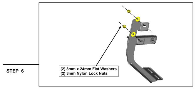
Loosely connect the (1) Driver Center step bracket to the (1) Driver Center reinforcement bracket using (2) M8 × 24mm flat washers, and (2) M8 nylon lock nuts.
