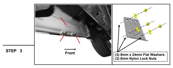
Start installation toward the front of the Driver/Left side of the vehicle.
