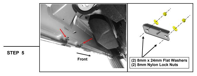
Loosely fit the (1) Driver Center reinforcement bracket to the (2) lower threaded studs using (2) M8  $\times$  24mm flat washers, and (2) M8 nylon lock nuts. Do not fully tighten to allow for later adjustments.
