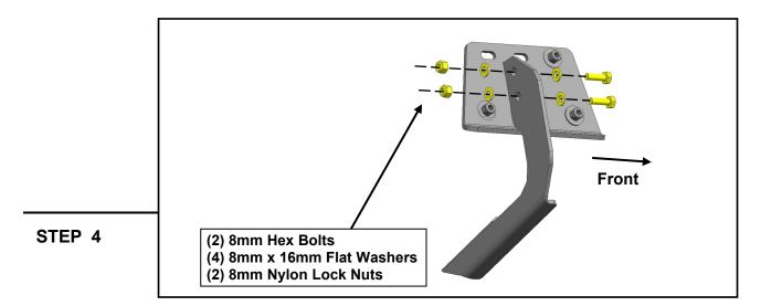
Loosely connect the (1) Driver Front step bracket to the (1) Driver Front reinforcement bracket using (2) M8 × 25mm hex bolts, (4) M8 x 16mm flat washers, and (2) M8 nylon lock nuts.
