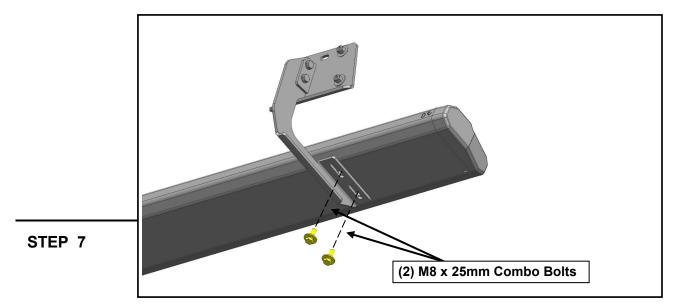
With all brackets loosely mounted to the vehicle, fit the Driver/Left Running Board onto the brackets, and loosely secure into place using (6) M8 x 25mm combo bolts.
