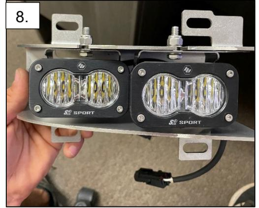
9. For initial fitment, center the light in the bracket leaving the same gap top to bottom. Rotate the light so the face is parallel to the mounting tab. For the outward light, do the same or face outward depending on preference.
