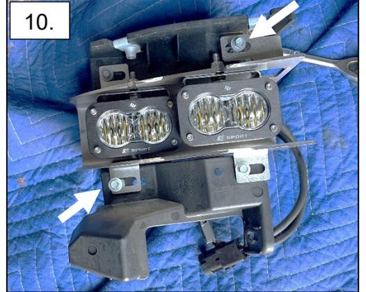
11. While checking alignment, rotate the lights to achieve the desired lighting. Use the slots in the steel bracket to shift the lights left to right to eliminate any unwanted gaps. Once the positioning is correct, tighten all hardware.
