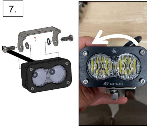
8. Using the supplied 1/4-20 hardware, mount the lights to both the driver side and passenger side brackets. (Note: The passenger side bracket is used for this photo)
