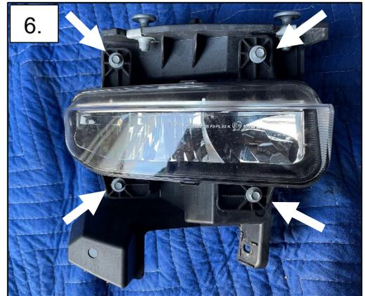
7. Assemble the standard bracket onto the light like the exploded view. If the bezel is as shown on the light, using a 2.5mm Allen wrench, remove the (4x) allen bolts and rotate the Bezel 180.
