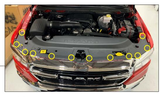
Open the hood. Remove (12) plastic push clips from the radiator support cover. Remove cover from vehicle.
