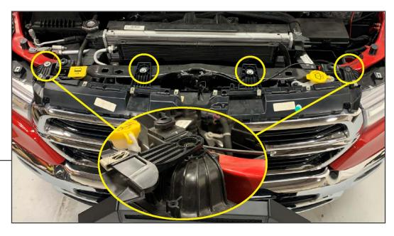
Remove (4) 10mm bolts from the top of the grille. Slightly lift the grille tabs over the bolt holes, then remove the grille from the vehicle.
