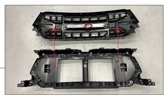
Transfer the OEM rear grille panel to the new grille, then press firmly to engage all the plastic retaining tabs. Secure the panel into the new grille reusing the original (10) 8mm screws.
