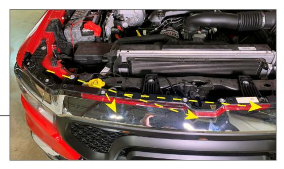
Re-install the headlight into the vehicle. Install the new grille into the vehicle using the original grille hardware. Plug in each LED light to the wiring harness. Neatly secure the harness inside the engine bay away from any moving/hot components.
