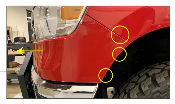
Remove (2) 8mm screws from the inner fender above the front bumper. Remove (1) 10mm bolt connecting the plastic panel to the fender. Peel the plastic panel outward from the fender, then pry the front of the panel away from the vehicle.
